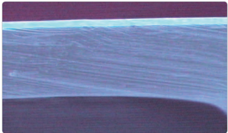
COEXTRUSION Coextrusion observed with a microscope.
