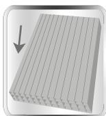
**ALWAYS PLACE THE SHEETS WITH THE AIR CELLS IN THE DIRECTION OF THE SLOPE**
