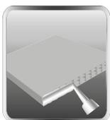
**ONLY USE POLYCARBONATE-COMPATIBLE SILICONE IF NECESSARY**
