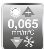
**ALLOW FOR THERMAL EXPANSION OF THE MATERIAL**
