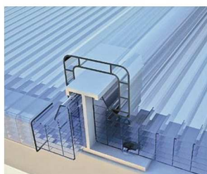
System with polycarbonate covergasket
