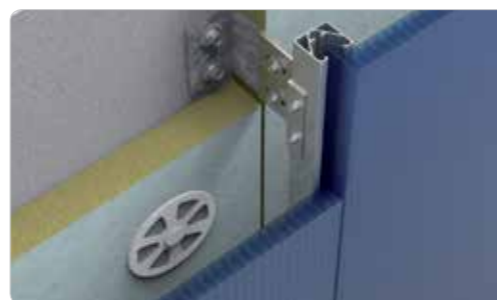
JUNCTION OF ADJACENT PANELS Paneling fixing to the masonry bearing wall, maintaining the cavity to fit insulation material and to allow air-circulation
