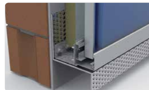
DETAIL OF CLADDING BASE INSTALLING Installation of profile 4271 to create facade base-support using panels th.20 mm
